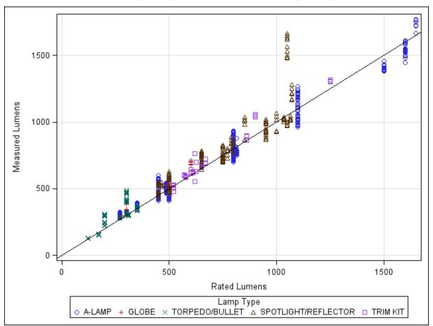
FIGURE 5-5: RATED LIGHT OUTPUT (LUMENS) VS. MEASURED LIGHT OUTPUT (LUMENS)
