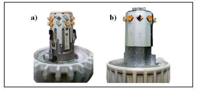
Figure 3-4. Two LEDs showing poor solder wetting on the gold pad.
