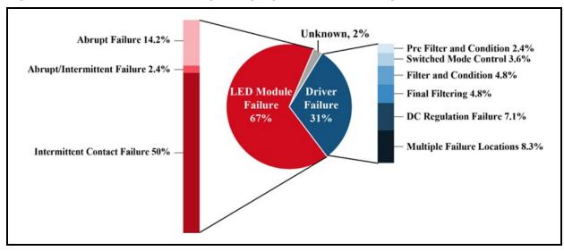
Figure 3-6. Failure location by category for test LED lamps.
