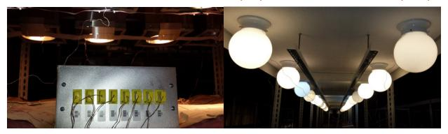
FIGURE 3-2: THERMAL TESTING IN RECESSED DOWNLIGHTS (LEFT) AND ENCLOSED CEILING FIXTURES (RIGHT)
